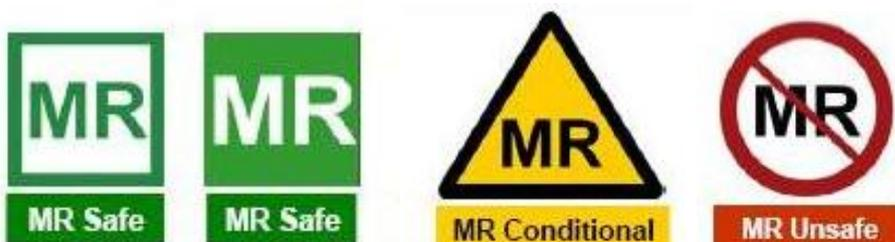
**MR safe** – defined as ‘an item that poses no known hazards resulting from exposure to any MR environment. MR safe items are composed of materials that are electrically nonconductive, non metallic, and nonmagnetic’
