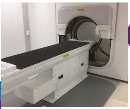
Figure 1: The MRI linac system being constructed in Manchester is nearing completion. The patient is placed in the bore of a 1.5T MRI, and the linear accelerator is rotating around the magnet. From a patient perspective, the linac is invisible, and imaging and radiation delivery can occur simultaneously.
