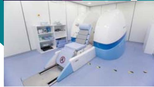
Figure 1: Bournemouth open, upright MRI scanner with table in the upright position and flexible spine coil in situ.
