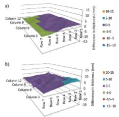
Fig. 7. Map of differences in thickness for the whole area for 18 cm  $\times 24$  cm nonflexible compression paddle for (a) Siemens Mammomat Inspiration, which had the smallest (3 mm) difference between measured and readout thickness across the whole area and (b) GE Senographe 800 T, which had the largest (7 mm) difference in measured and readout thickness across the whole area, when applying 100 N compression force.
