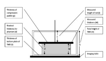
Fig. 5. Diagram to illustrate the measurements performed to calculate readout and measured thickness of the object
