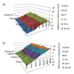
Fig. 6. Map of differences in thickness for the whole area for 18 cm  $\times$  24 cm flexible compression paddle for (a) Hologic Selenia Dimensions, which had the smallest (12 mm) difference in thickness across the whole area and (b) Hologic Lorad Selenia, which had the largest (19 mm) difference in thickness across the whole area, when applying 100 N compression force.
