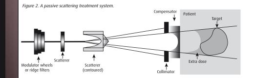
Figure 3. Individual collimator and compensator used in passive scattering proton systems.
