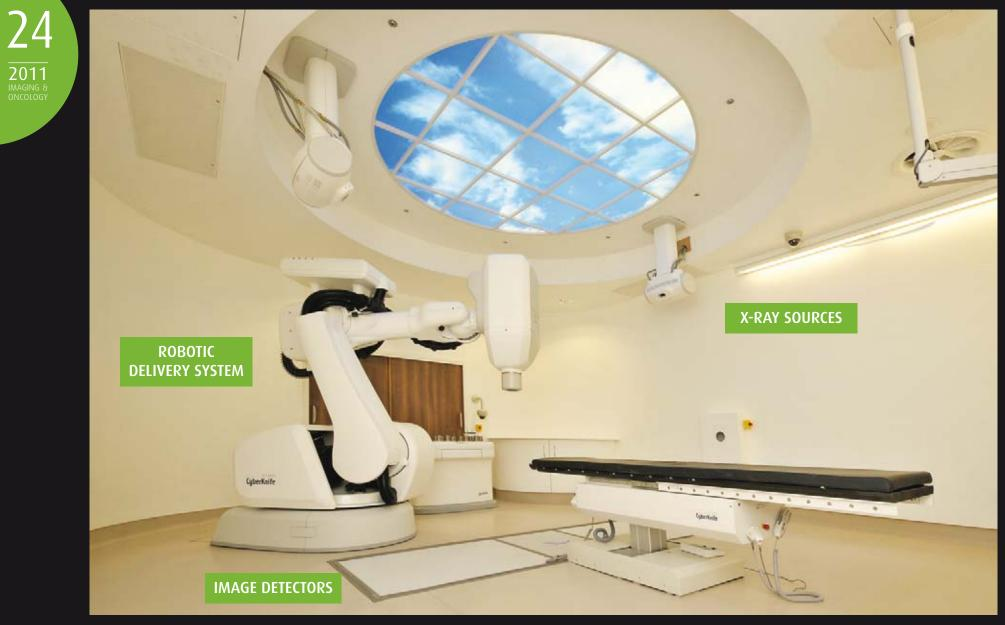
Figure 1. CyberKnife robotic delivery system
