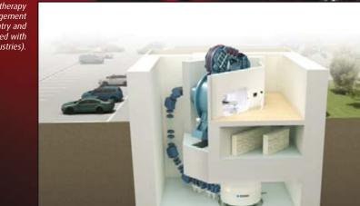
Figure 6. a) A new proton radiotherapy system designed in a vertical arrangement with a compact type rotating gantry and a 230MeV cyclotron (reproduced with permission from Sumitomo Heavy Industries).
