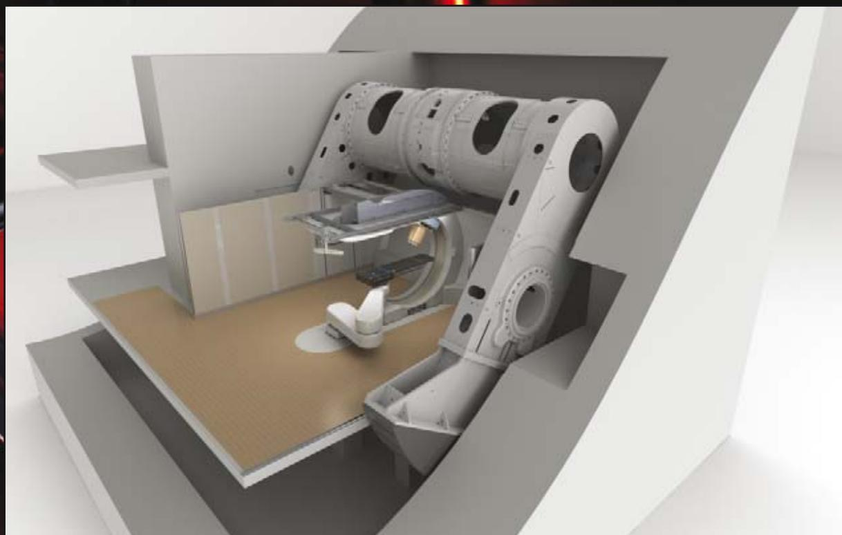
b) A single room proton facility designed with a rotating cyclotron (reproduced with permission from Still River Systems).
