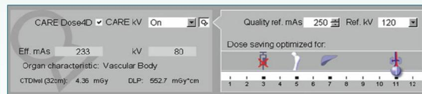
Figure 1. Shows CARE kV turned ‘On’, with the dose saving optimizer bar set to 11. (Yu, Fletcher and McCollough, 2010).
