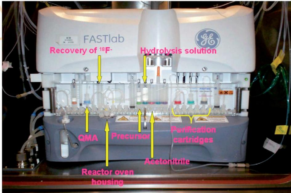
Figure 2: An example of an [<sup>18</sup>F]FDG module equipped with cassette: Fastlab GE
