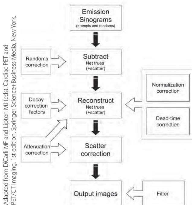
Figure 4: Flowchart for PET image processing and reconstruction
