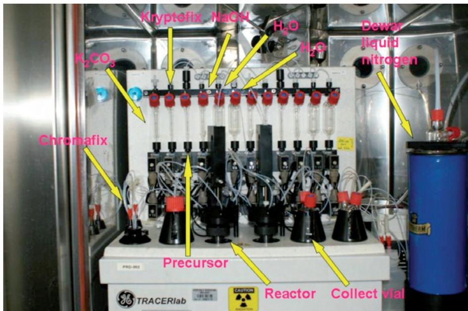
Figure 3: An example of an [<sup>18</sup>F]FDG double module: TRACERlab FX GE
