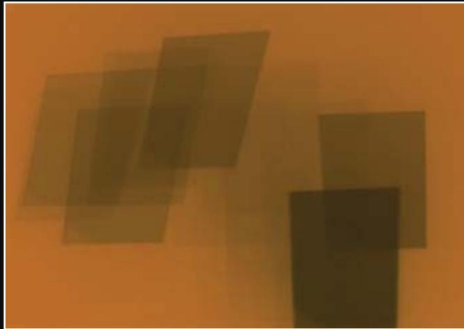
Figure 1: Example of radiochromic film demonstrating exposure areas correlating with peak skin dose.
