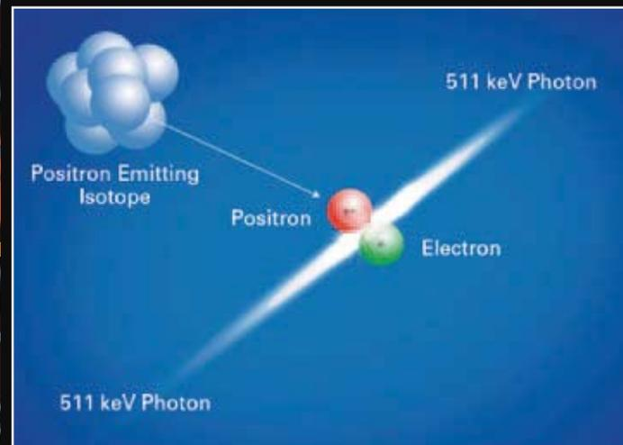
*Figure 1: The principle of positron 'emission' involves a positron (+ve charge) being emitted from an unstable isotope. Within moments of positron emission (a distance of ~ 1mm) it is attracted to an electron (-ve charge). The positron and electron are attracted with such force they 'annihilate' and 511 KeV photons (gamma rays) are emitted in opposite directions at almost 180°. It is this principle which forms the basics of PET physics.*
